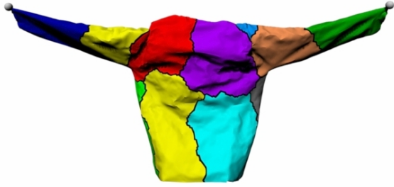
Figure 4: Partitions of a mesh shown in different colors for 12 processors.
