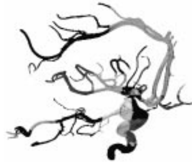
Figure 3: Octree decomposition of reconstructed vessel tree. Different grey-shades mark geometry of different octants.
