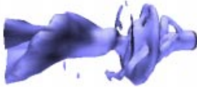
Fig. 7. Vortex breakdown of a fluid which is injected in another fluid.
